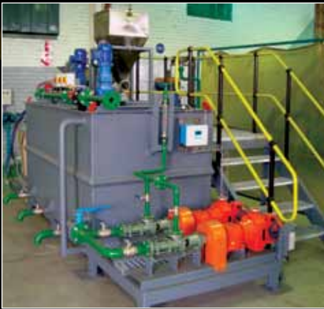
MIP-200 Flocculant Plant
