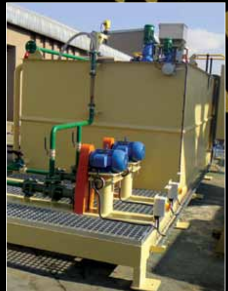
Skid mounted Flocculant Plant
